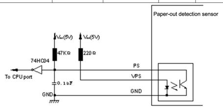
PS signal will be high level when run out of paper
